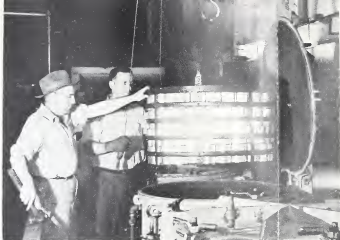
Canned sweetpotatoes go into a pressure vat for processing. It takes a great deal of planning and work before the food grown by the farmer gets to city consumers in a form they can use. 8311
